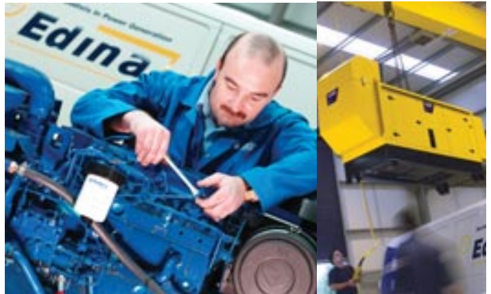
Servicing a small diesel generator and loading a larger standby generator at Edina.
